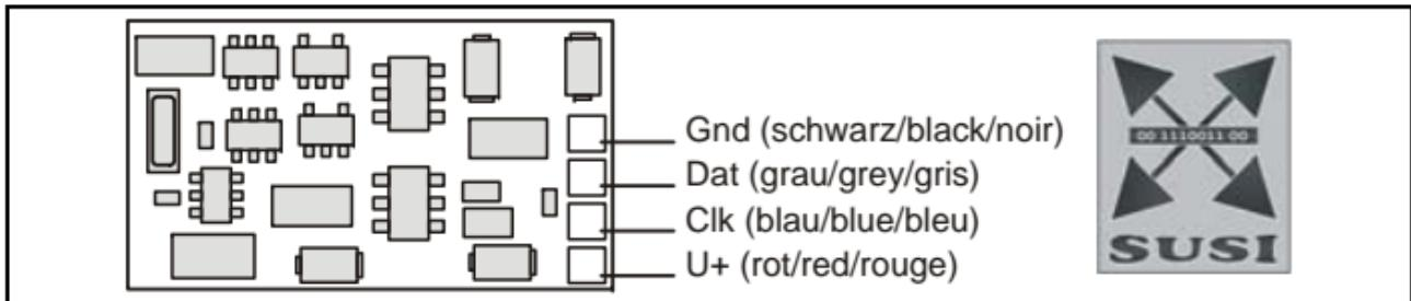
Abb. 2: S.U.S.I. – Schnittstelle / S.U.S.I. interface / Interface S.U.S.I.
