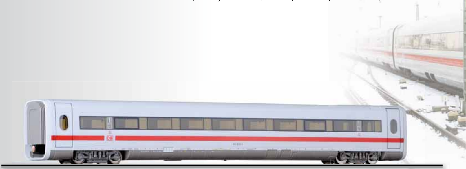
ICE 1-Ergänzungswagen 1. Klasse der DB AG 1st class passenger coach of the DB AG, additional to ICE 1
